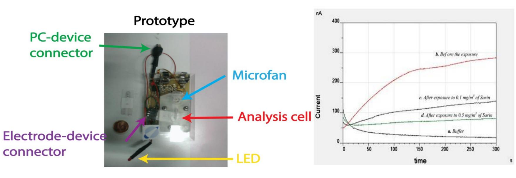
**Fig. 5** (Left) image of the prototype, (right) original recording obtained using a biosensor in 0.05 M phosphate buffer solution + 0.1 M KCl, pH 7.4. Applied potential + 200 mV vs Ag/AgCl. Signal recorded in phosphate buffer (a) and in a solution of butyrylthiocholine (5 mM) before the exposure of the biosensor to sarin gas (b) and after 1 min exposure to 0,1 mg m<sup>-3</sup> (c) and to 0.5 mg m-3 (d) of Sarin gas.
