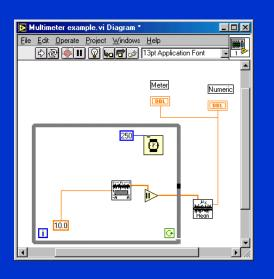
Example 1: Analog & Digital Voltmeter (*simulated signal*)
