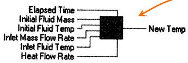
the <u>connector</u> defines the inputs and outputs
