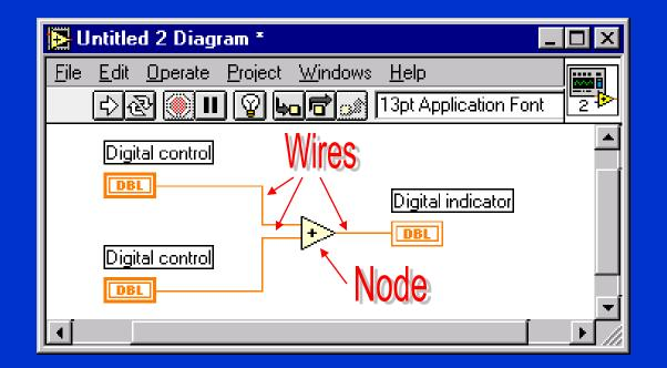
A LabVIEW VI is held together by <u>wires</u> connecting nodes and terminals; they deliver data from one source terminal to one or more destination terminals.
