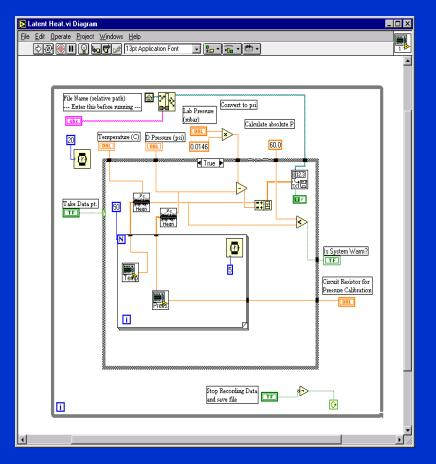
The *block diagram* window holds the graphical source code of a LabVIEW VI – it is the actual executable code
