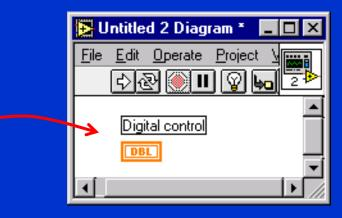
LabVIEW automatically creates a corresponding <u>control</u> (or <u>indicator</u>) <u>terminal</u> on the BLOCK DIAGRAM
